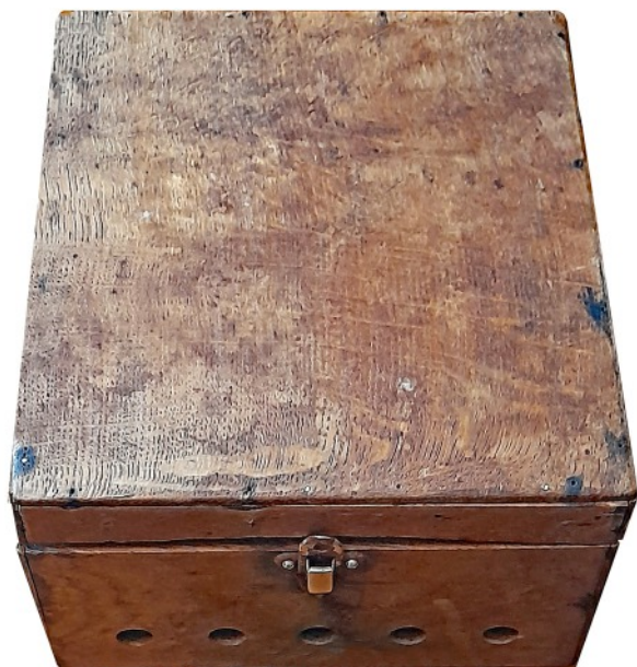
Five ventilation holes were included in the front side of the oak enclosure, which was rather flimsy, but still strong enough considering the examples that survived.
